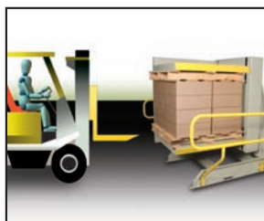
2. Place loaded pallet into inverter.
