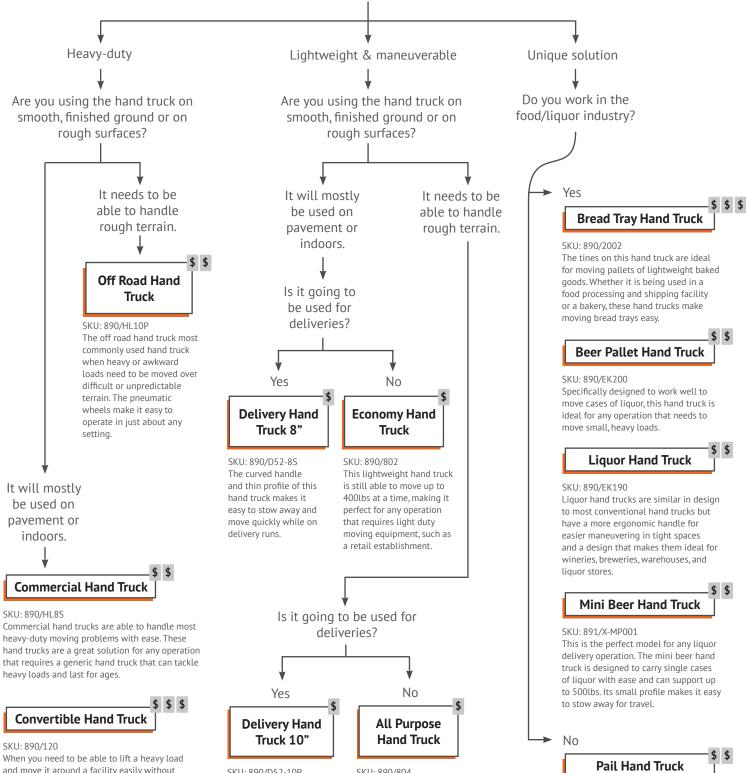
When you need to be able to lift a heavy load and move it around a facility easily without worrying about it tipping, it is worth considering a convertible hand truck. The ability to turn your hand truck into a cart makes moving cargo long distances much easier.
